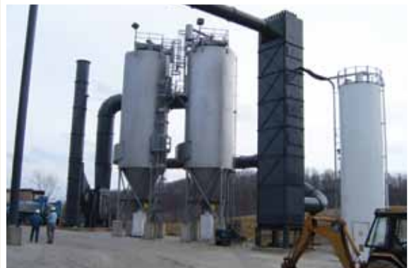
484RF two high temperature collectors on secondary aluminum processing
